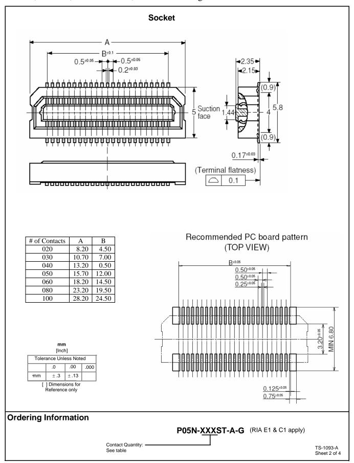
0.5 mm, Vertical, Surface Mount, 3 mm Stack Height
